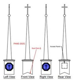
To the left is what our steeple will look like. The "blue", octagon panels will actually be a frosted look of clear glass - the blue is just the company's drawing. The octagon panels will be on the west and east sides. The front will be blank, and the back has an access panel that doesn't show.
